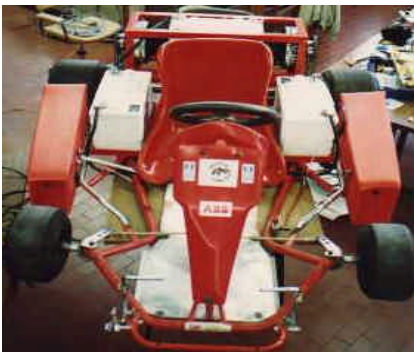
Fig. 2: Electrical kart with two independent wheels drives
